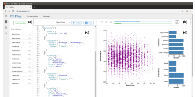
Fig. 10. P5 Play allows users to progressively analyze multidimensional data using declarative visualization grammars. P5 Play’s user interface consists of a side panel (a) for selecting data files and listing the data attributes, a control panel (b) for starting and pausing progressive operations, a text editor (c) for editing declarative specifications, and a dashboard (d) for displaying the output visualizations.
