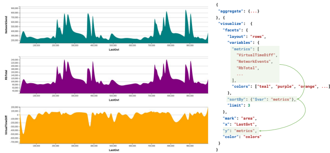
Fig. 6. Declarative specification for visualizing multivariate time-series data in faceted views showing the top 3 user-defined variables ordered by their variances.
